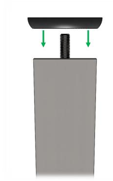
Step #2 - Place the linkplate on top of the leg.
